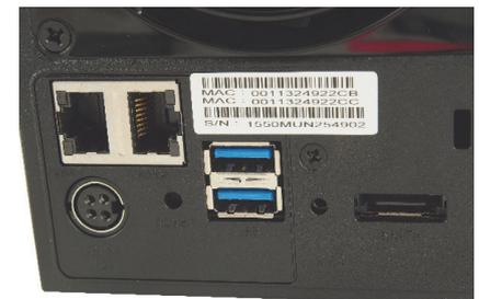
Dual connections for redundancies, as well as the e-Sata port for expandability
