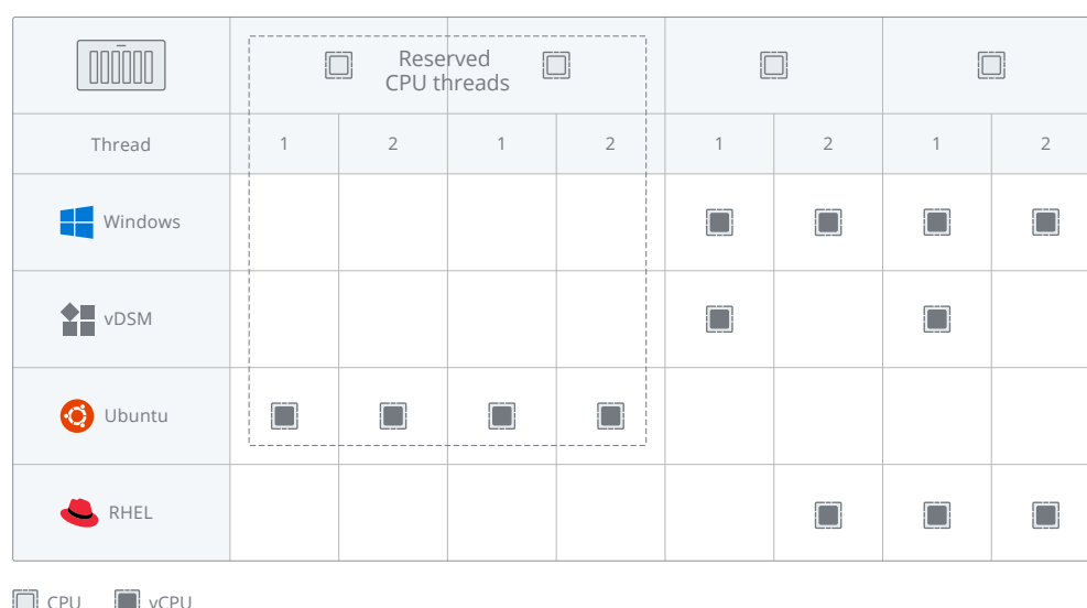
Figure 4: In this example, four CPU threads on two physical CPU cores are reserved for one Ubuntu Linux VM, while Synology VMM divides the other vCPUs over four remaining non-reserved threads based on relative load. Users can specify the number of vCPUs they wish to assign to each VM and whether these are to share physical CPU resources, or run on reserved CPU threads. Virtual Machine Manager automatically balances loads between non-reserved CPU threads.
