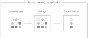
ActiveProtect uses a unique identification method to classify and manage backup data, as part of its deduplication method. The backup data is divided into 4 KB chunks. Each chunk is assigned a unique fingerprint which is generated with the SHA-256 algorithm to ensure data integrity and uniqueness.
