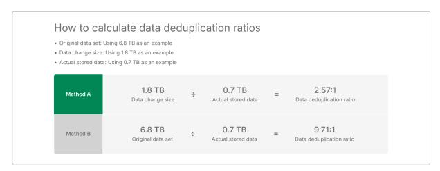
With **Method A**, only 1.8 TB of data is changed in size as the redundant data is removed through CBT and then further compressed so that there is a total of 0.7 TB of data that is to be stored at the backup destination.
